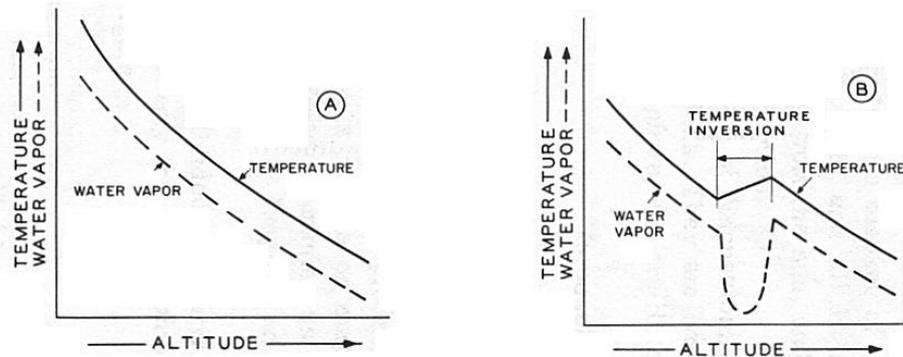
**LONG DISTANCE TROPOSPHERIC PROPAGATION** takes place because of temperature inversion. Normal temperature and water vapor content of air decrease with altitude (A). Refractive index of the atmosphere can produce inversion area (B), showing an abrupt break in water vapor content. If the inversion is pronounced, the resulting bending of the radio wave will follow the curvature of the earth. Atmospheric ducts have propagated VHF signals over distances in excess of 2500 miles.
