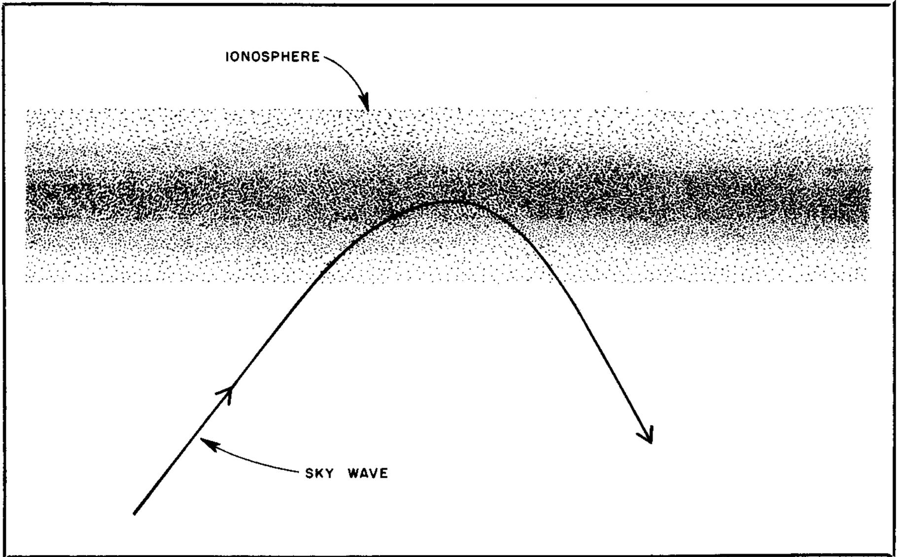
Fig. 2 — Under proper conditions, a radio wave entering the ionosphere will be refracted and follow a new course. This permits the signal to be heard on earth, perhaps thousands of miles from the transmitting antenna.
