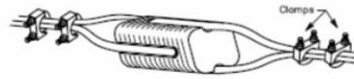
Fig 10—Stranded guy wire should be attached to strain insulators by means of standard cable clamps made to fit the size of wire used.
