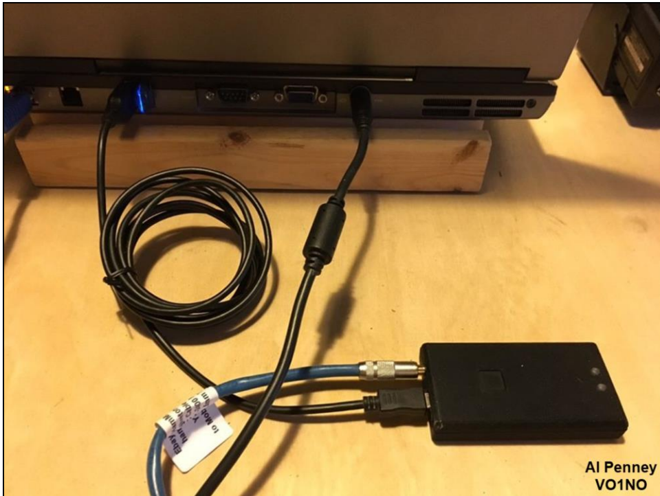
Portable APRS gateway station we use for tracking high altitude balloon launches by the Annapolis Royal Space Agency. The small box is the TNC,
