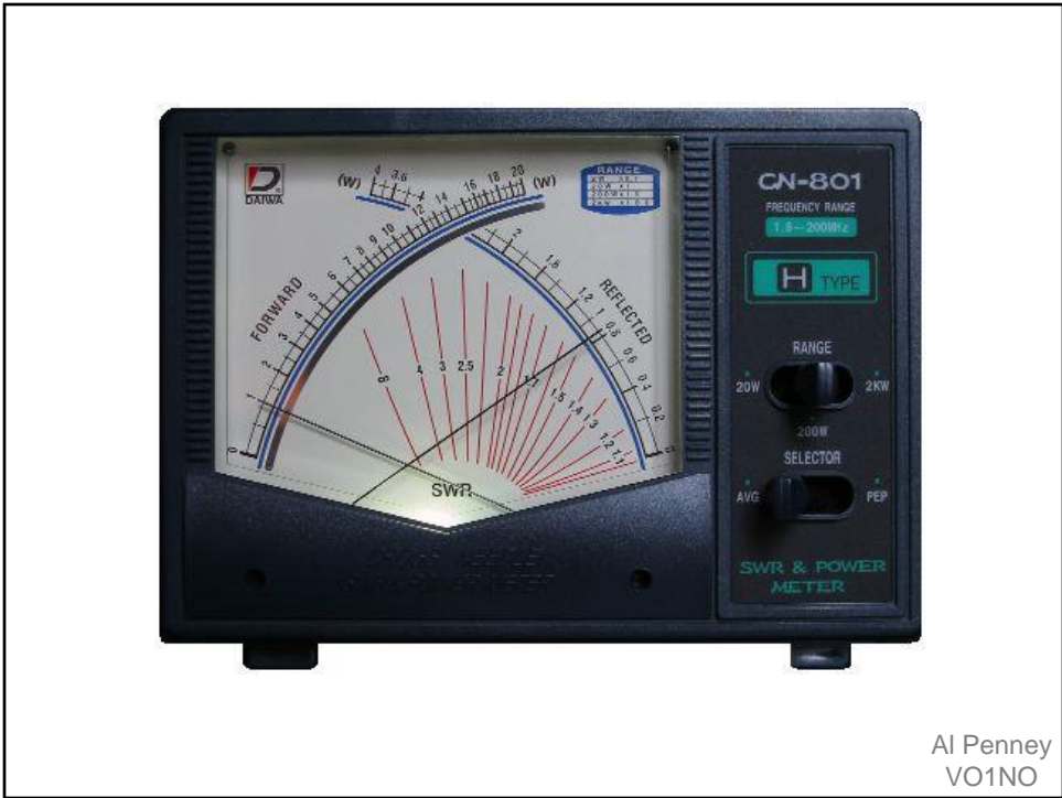
Power SWR meter, using crossed needles.
