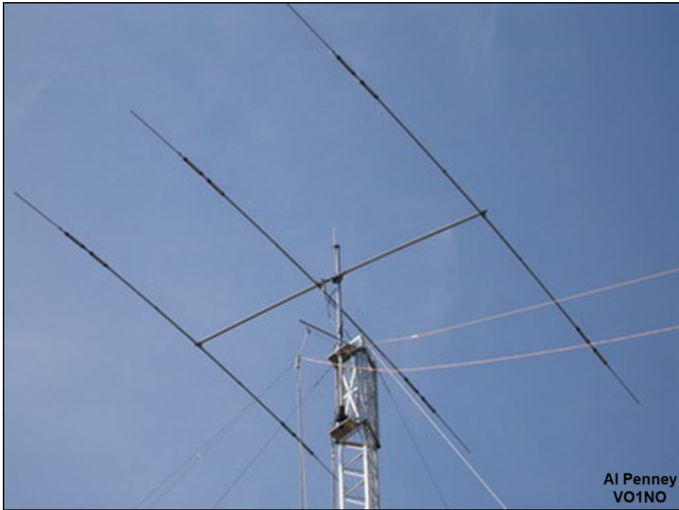
Three element Triband antenna (covers 10, 15 and 20 meter bands).
