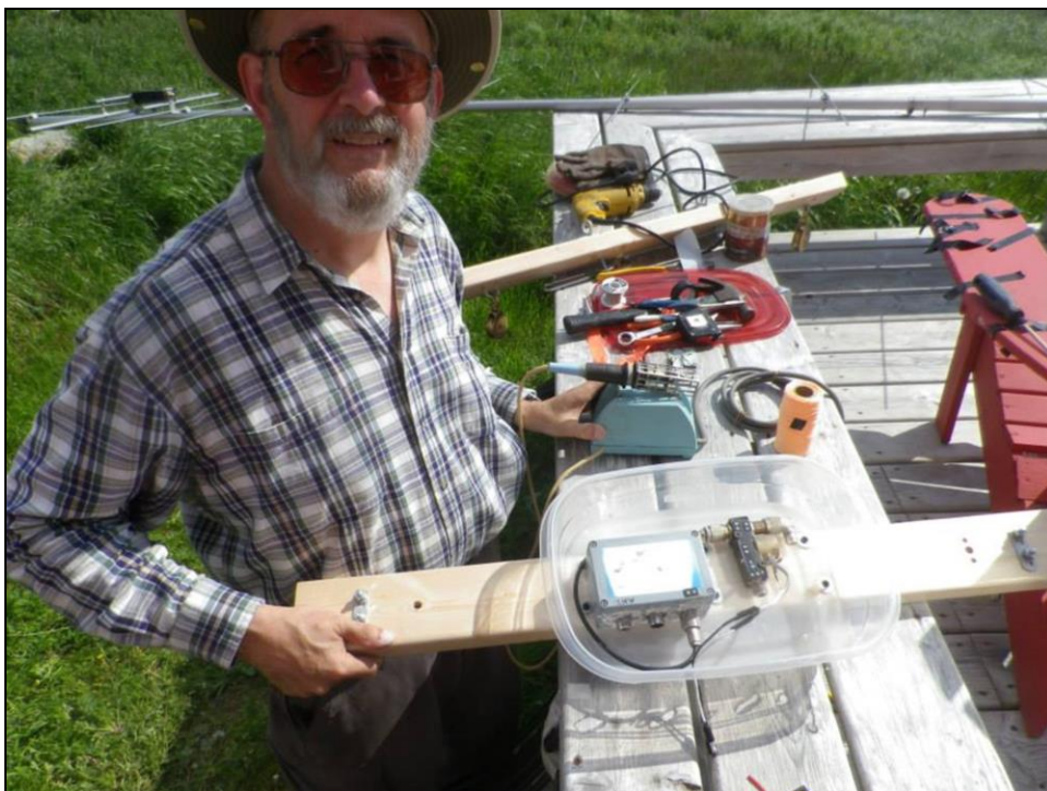
Fred VE1FA assembling the receive preamplifier and associated relays at the rope yagi's feedpoint.
