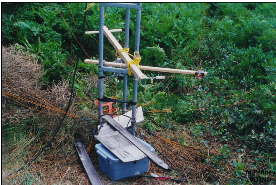
Feedpoint for shunt-fed tower. Capacitors in Rubbermaid container.
