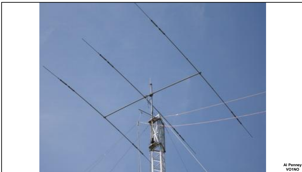
Three element Triband antenna (covers 10, 15 and 20 meter bands).
